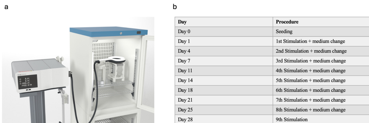
Figure 1. Experimental setup and protocol. (a) Experimental setup used in our study. The control and stimulated groups were placed identically in the incubator with the EMTT device turned on for the stimulated group and kept off for the control group. (b) Stimulation protocol used in our study. The day of stimulation and medium change are illustrated.
